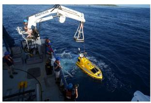
Autonomous sonar vessel being launched from *Nautilus*
